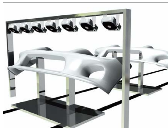
Neutralization and dust removal of molded bumpers before painting process
