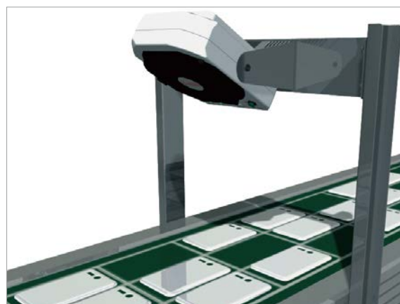
Dust prevention on molded parts
