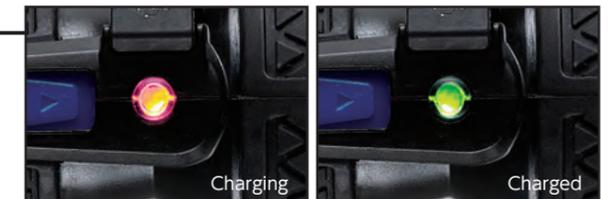
\* For circuit-board protection, the lamp of the 220USB flashes red and the screwdriver stops operation, when a load such as 2N·m or over is given during electric-powered use. If the charge level of the battery is less than 15%, the battery charge lamp will flash red during operation.
