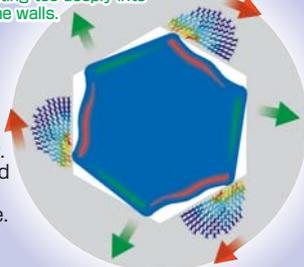
Radius part of this unique "UltraHex" bites Hex screw A/F to thrust for turning power. Automatically this unsurpassed driving mechanism controls smooth and high driving torque.
