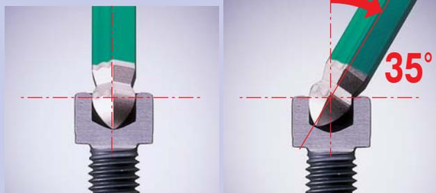
The driving part of "RainBall" is designed to fit the hex hole at a high position, making it possible to tighten screws at a 35-degree angle. The pointed tip becomes the center of smooth power rotation.
