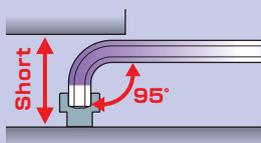
95° short hand gives easier operations. Ideal for tightening screws at a narrow space.
